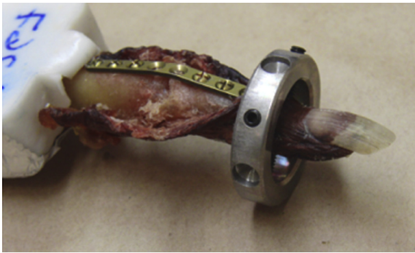
FIGURE 6: PIP joint arthrodesis using dorsal plate fixation. A load-application device, consisting of a metal ring with 4 cavities to host the end of the rod, was fixed with 4 screws to the shaft of the middle phalanx 20 mm from the PIP joint.
