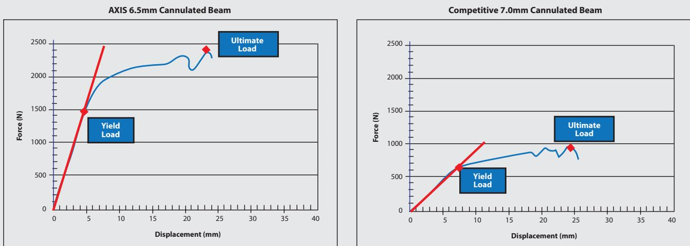
Figure 7: The red line represents the calculated stiffness (N/mm). Note: the 6.5mm Axis beam has a 182% increased yield load, and 150% increased ultimate load over the 7.0mm competitive beam.
