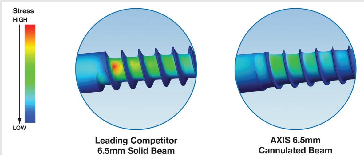
Figure 10: Finite element analysis of AXIS 6.5mm cannulated implant and the competitive 6.5mm solid implant showed a significant reduction in surface stress for the AXIS cannulated beam. Red indicates area of a potential stress riser at the thread transition from the shaft.
