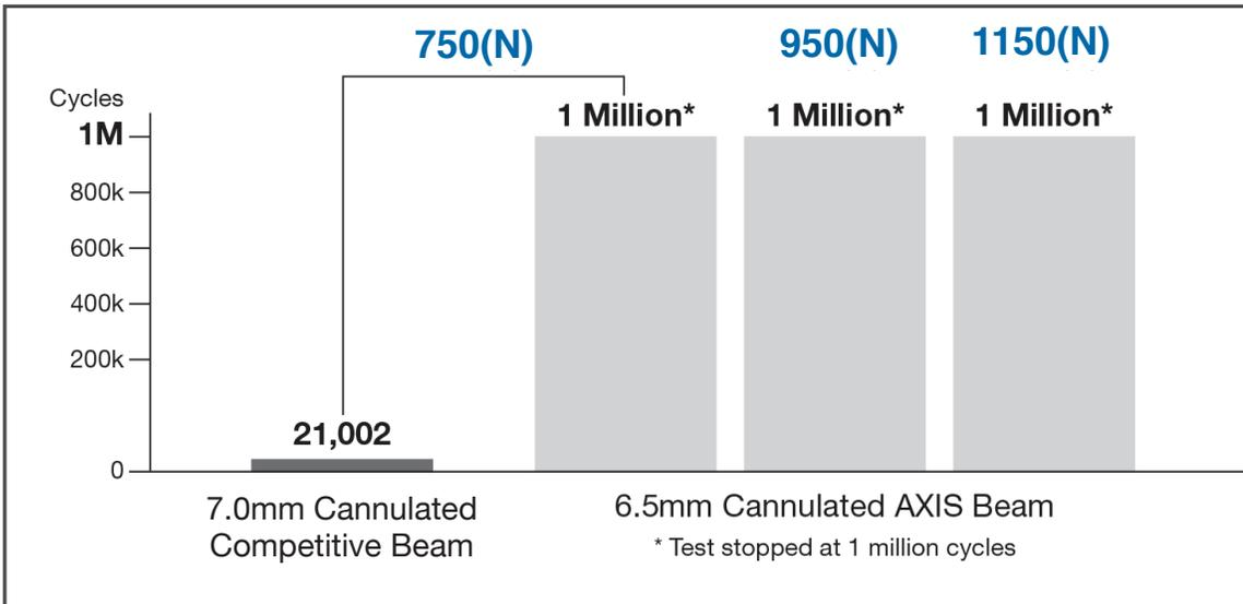
Figure 8: The AXIS beams demonstrated forty-seven times more the fatigue life than the competitive beams at 750(N). The AXIS beams also survived 1,000,000 cycle runouts at higher loads: 950 (N), and 1,150 (N).
