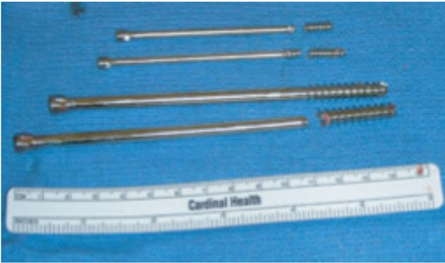
Figure 5: Broken Competitive headless compression screws retrieved from a patient with non-union and recurrence of deformity following beaming. Note that the three broken screws failed at the predicted stress riser near the thread transition from the shaft
