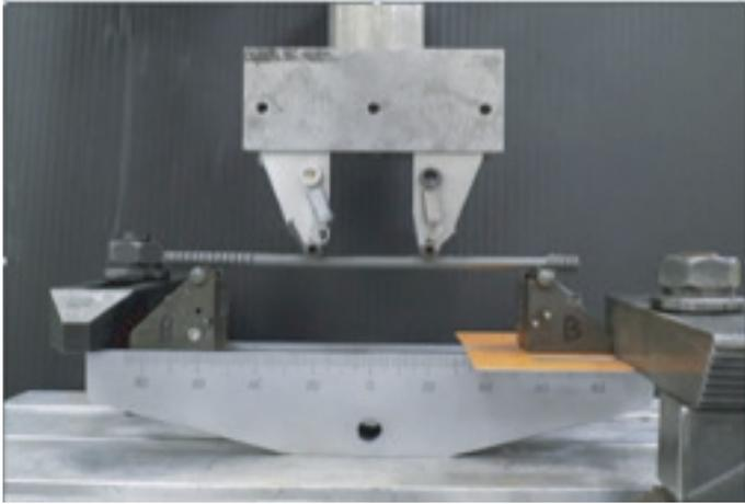
Figure 9: Example of the 4-point bending apparatus utilized for both static and dynamic bending tests between the AXIS system and the competitive system. Dimensions for inner loading distances and outer support distances are consistent with ASTM F382-17.
