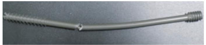
Figure 9a: Example of fatigue fracture of 7.0mm competitive beam @ 21,000 cycles (750 N).
