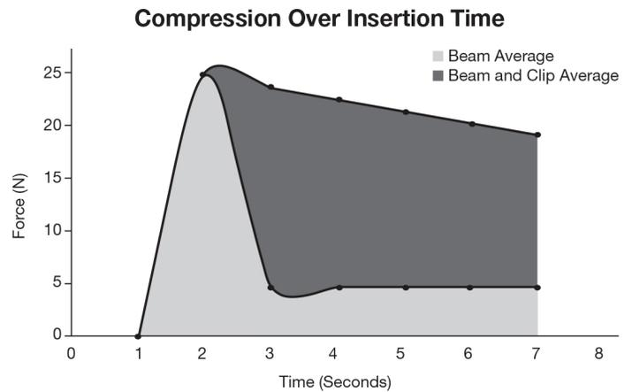
Figure 12: Illustrates the X-Clips ability to maintain compression with the advancement of the beam. The AXIS beam/X-Clip construct essentially acts as a "nut & bolt" and limits screw strip-out.
