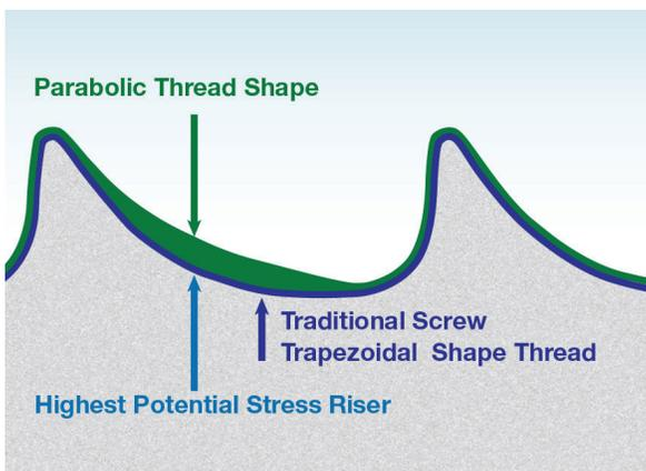
Figure 6: AXIS parabolic thread shape compared to traditional, third generation beam thread pattern. More material is present in the leading edge of the thread reinforcing the area where the greatest stress occurs.
