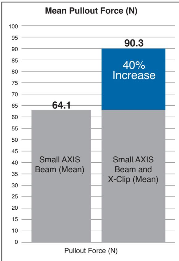
Figure 11: Axial pullout forces for the AXIS beam system when used with and without the X-Clip supplementary fixation device. Note: The AXIS beam/ X-Clip construct provided 40% additional pull-out strength versus the beam alone
